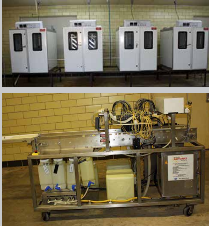
Incubation research and in OVO vaccination; four 1080 egg & two 5000 egg incubators (provided by Chickmaster).
